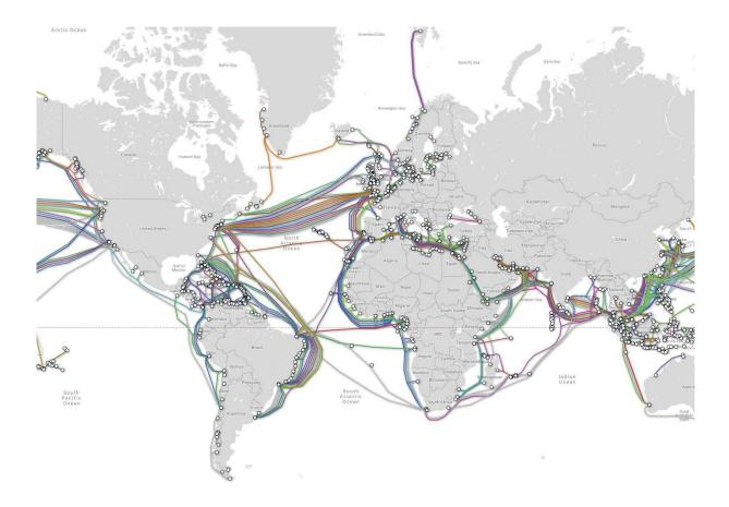
Map of fiber optical cables on the seabed. These cables are transporting 99~% of all transoceanic digital communication.
